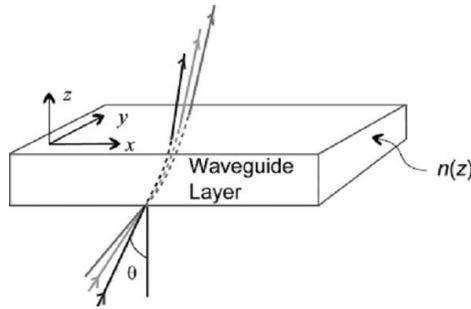
Figure 2: Experimental setup: a set of sampling rays propagating across the waveguide layer
