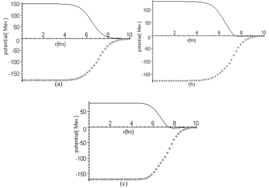
Figure 1: The real and imaginary parts of equivalent local potential,  $U_L$ , for  $\pi^- + {}^{208}_{82}\text{Pb}$  at  $a : 162(\text{MeV})$ ,  $b : 180(\text{MeV})$ ,  $c : 291(\text{MeV})$  energies. The continuous curves are the real part and the square shape curves are the imaginary part of the potential
