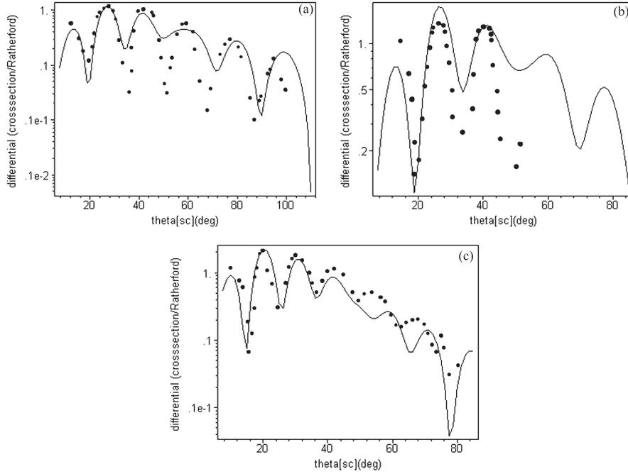
Figure 2: Elastic scattering differential cross-section of negative pion, continuous curves, from  $^{208}_{82}Pb$  target using equation (14) at  $a : 162(MeV)$ ,  $b : 180(MeV)$ ,  $c : 291(MeV)$  energies. Data points are from references [10], [4], and [3] respectively
