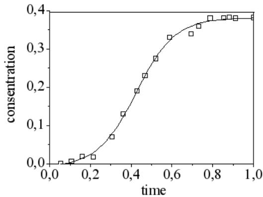
Figure 5: Dimensionless oxygen concentration profile in liquid phase in time ( $K_La = 0,0753$ ,  $L = 2m$ , without biomass); (—) – the model solution; (□) – experimental data (desalt water)
