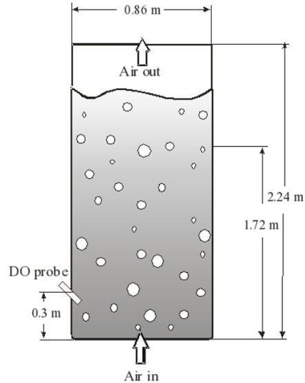
Figure 1: Bubble column experimental set-up
