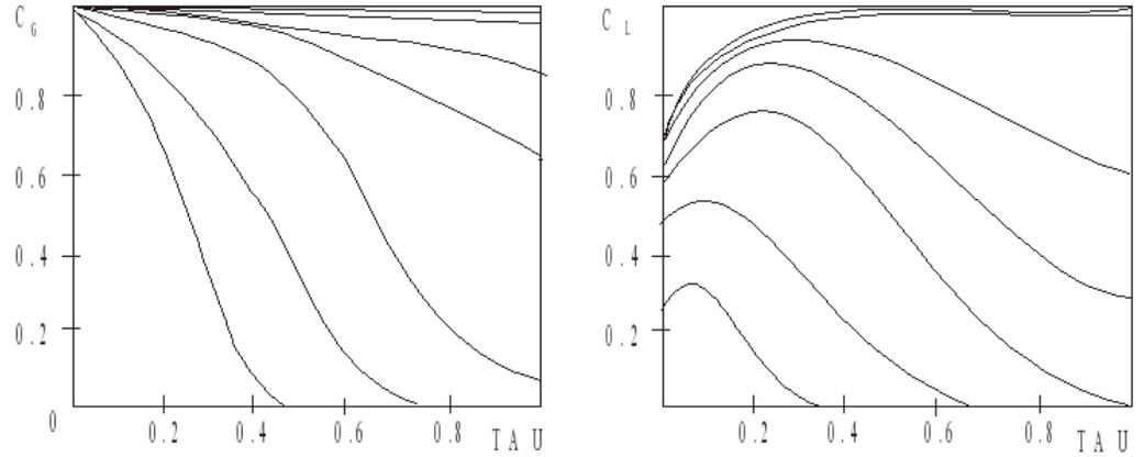
Figure 3: Dimensionless profiles of oxygen concentration in gas and liquid phases along the fermenter in conditions, used by Shioya and Dunn
