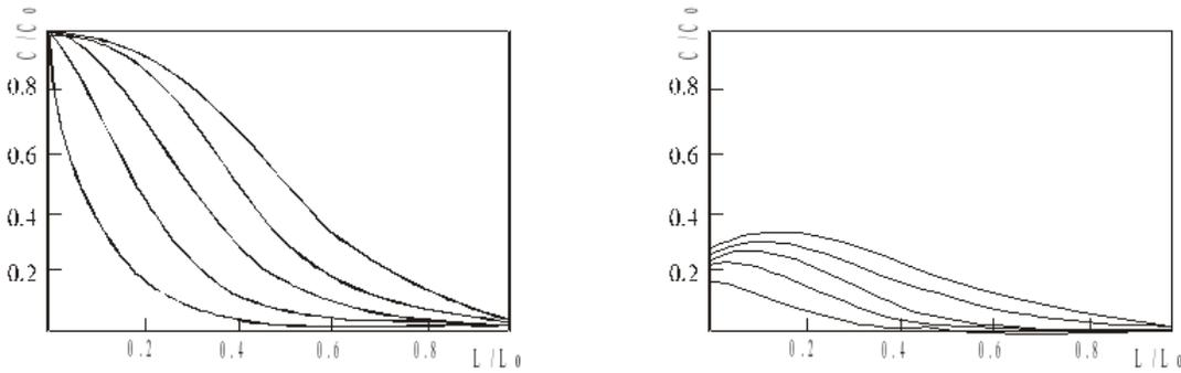
Figure 2: Dimensionless profiles of oxygen concentration in gas and liquid phases along the fermentor – numerical results for five steps in time ( $K_{La} = 0,0693$ ,  $L = 10\text{m}$ , without biomass)
