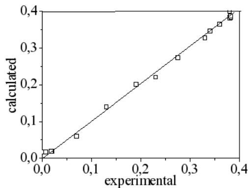
Figure 6: Comparison between the model solution and normalized experimental data. The  $U_G$ ,  $U_L$  and  $K_La$  have been estimated as it is referred above
