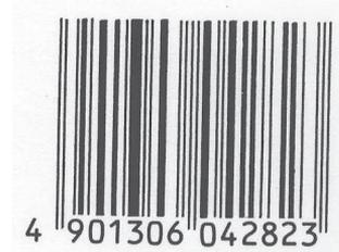
smallest multiple of 10 larger than 67 is 70, and subtracting 67 from 70 yields  $70 - 67 = 3$ . The check digit is therefore 3. Owing to this check, the ratio of correctly read-in barcodes is kept high.
