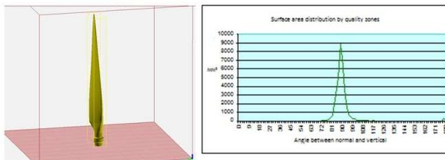
**Figure 4:** Blade with a vertical arrangement in the printer's chamber and the distribution of its areas along the normal to the vertical
