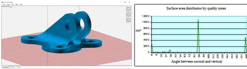
**Figure 5:** The horizontal arrangement of the bracket and the diagram of the distribution of areas by zone. The proportion of areas in areas of poor quality is 14%
