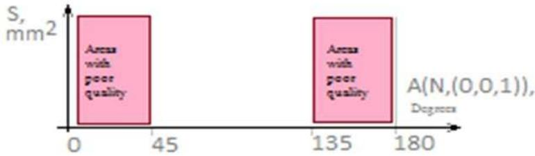
**Figure 2:** Zones with poor surface quality in the distribution diagram of areas by the angle between the normal and the vertical
