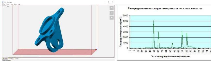
**Figure 6:** Optimum in terms of the quality of the surfaces of the arrangement of the bracket and the diagram of the distribution of areas by zone. The share of areas in areas of poor quality is 12%
