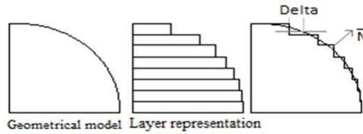
**Figure 1:** The difference (delta) between the geometry of the layered representation and the original bypass, depending on the normal ( $N$ ) of the surface
