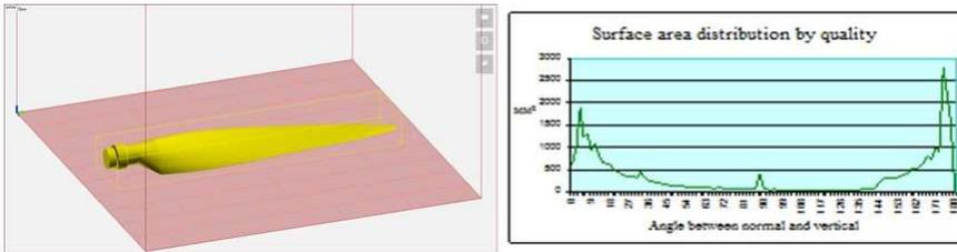
**Figure 3:** Blade with a horizontal location in the printer’s chamber and the distribution of its areas along the normal to the vertical
