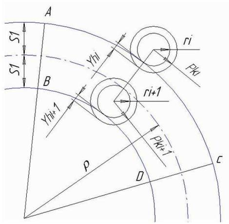
Figure 2: The Scheme to the Calculation of Slipping Wheels out of the Wage Wheels Towards the External and Internal Rails in the Curved Section of the Track
