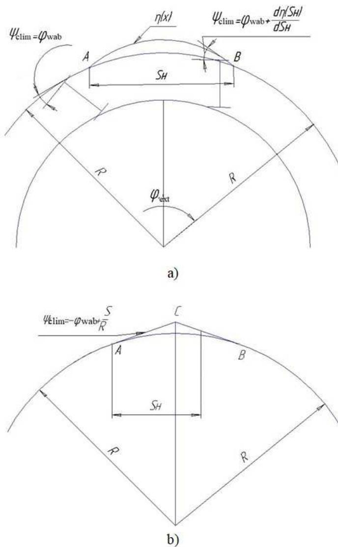
Figure 1: Scheme to the Definition of the Angle of Wage Wheels Climbing on the Isolated Inequalities in the Plan along the External Rail of Circular Curve: a) on Smooth Surface; b) on Conjunction ("Angle") Inequality in the Rail Conjunction.
