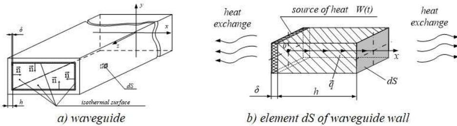
Figure 2: Design model of heat transfer at a waveguide wall
