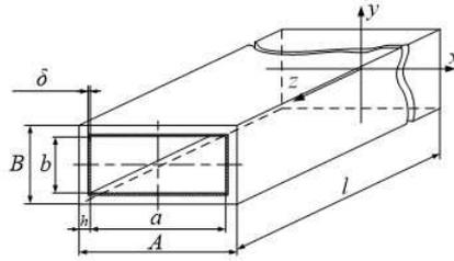
Figure 1: Design of a waveguide straight section
