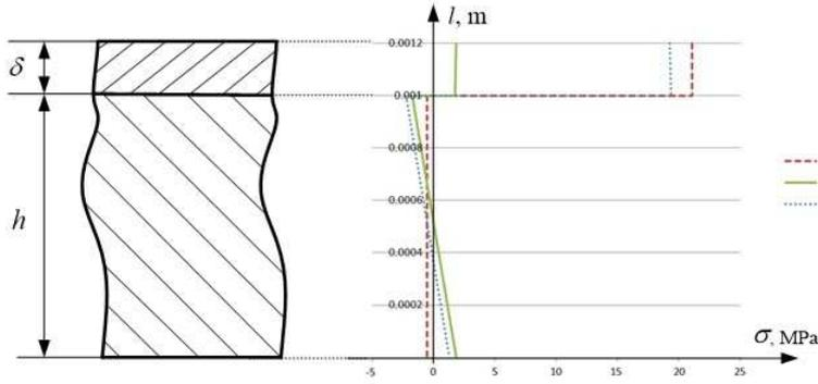
Figure 4: Stressed state of a conductive coating
