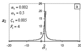
Figure 1a: Effects of the damping coefficient  $\zeta_2$
