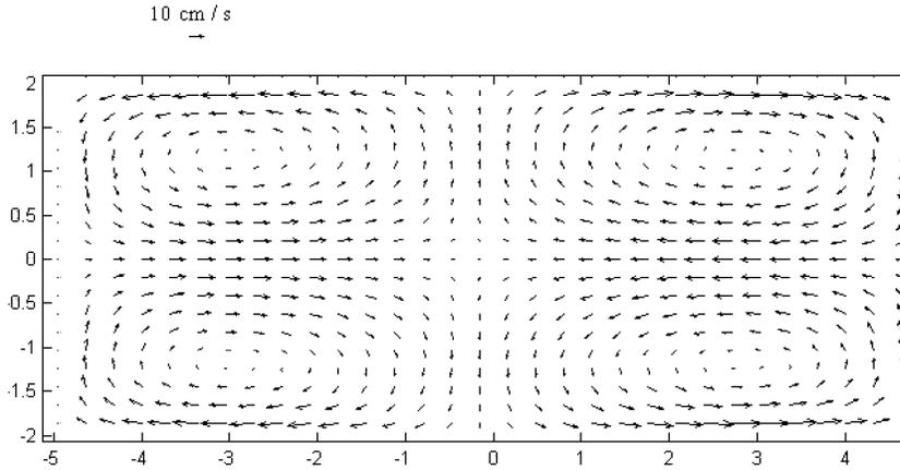
Figure 1: Velocities calculated using the presented vorticity-stream function numerical approach at a layer 12 cm from the bottom in a 208 KA cell
