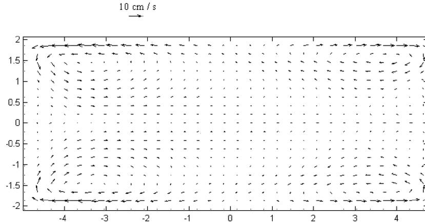
Figure 2: Velocities calculated using the proposed analytical technique at a layer 12 cm from the bottom in a 208 KA cell
