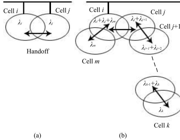
Figure 3: The arrival rates of the cells in: a) today's Wi-Fi network and b) infrastructure Wi-Fi mesh networks.
