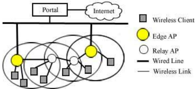
Figure 2: The topology of infrastructure Wi-Fi mesh networks
