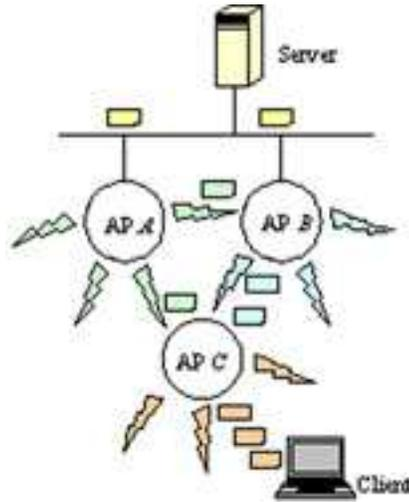
Figure 4: Frame duplicated during broadcast transmission in infrastructure Wi-Fi mesh networks
