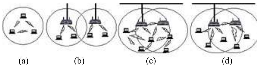
Figure 1: The system architectures of: a) IEEE 802.11 ad-hoc network, b) IEEE 802.11 infrastructure network, c) wireless mesh networks and d) Infrastructure Wi-Fi mesh networks
