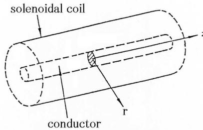
Figure 2: Solenoidal coil with unlimited length
