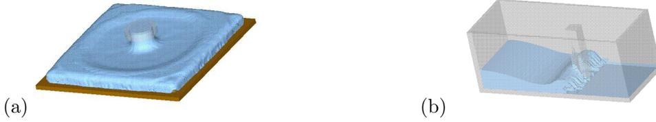
Figure 3: Numerical simulations of free surface flows at high Reynolds number: (a) Hydraulic jump at Reynolds 100; (b) Fluid structure interaction at Reynolds 99000
