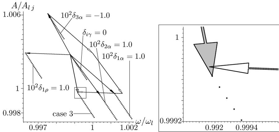
Figure 3: Influence of nonlinearity and physical inhomogeneity on the resonance frequency (case 3,  $j = 1, \dots, 20$ )
