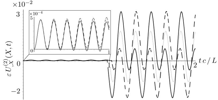
Figure 1: Influence of variable linear elastic properties on the nonlinear oscillations at the boundaries  $X = 0$  (*bold solid line*) and  $X = L$  (*dashed line*) of the material. *Solid line* - homogeneous material. The inset shows the solution in the interval  $0 < tc/L < 1$  with amplified ordinate
