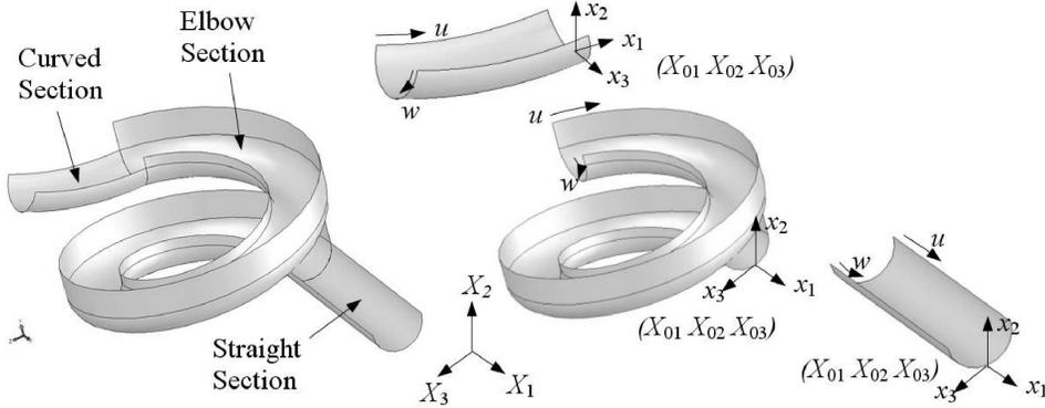
Figure 1: Geometric representation of waterslide in flume sections
