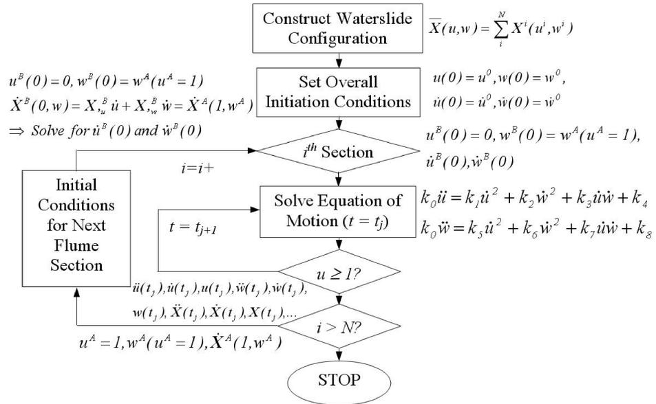
Figure 3: Computation flow for solving the equation of motion
