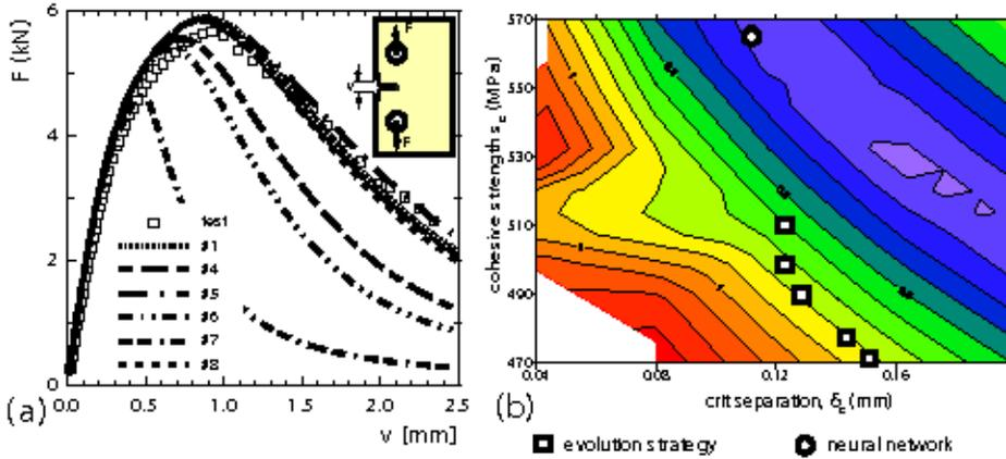
Figure 1: Force vs. displacement of a Kahn specimen; comparison of test and simulation results (left); Iso-contours of the error in the plane of the cohesive parameters,  $\sigma_c$  and  $\delta_c$  (right)
