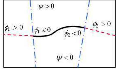
Figure 1. Nodal enrichment in XFEM      Figure 2. Crack representation using LSM
