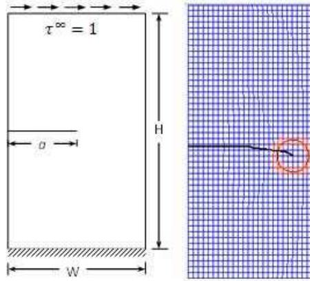
Figure 3. Edge crack under shear
