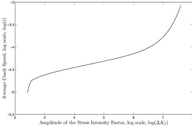
Figure 4: Dependence of  $\ln \hat{v}$  on  $\ln \Delta K_I$  predicted by the model
