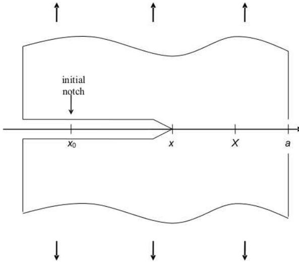
Figure 1: Specimen-loading configuration to be considered
