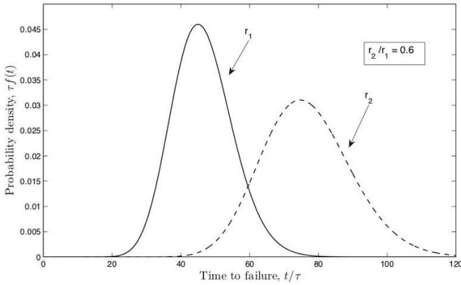
Figure 3: Probability density  $f(t)$  of time to failure for two values of  $r$ :  $r_1/a = 0.05$  and  $r_2/a = 0.03$
