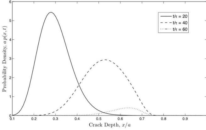
Figure 2: Probability densities of crack depth at various times. Not shown are the two atomic probabilities, one at  $x = x_0$  and another at  $x = a$ ,  $P(x_0, t)$  and  $1 - P(a, t)$ , respectively
