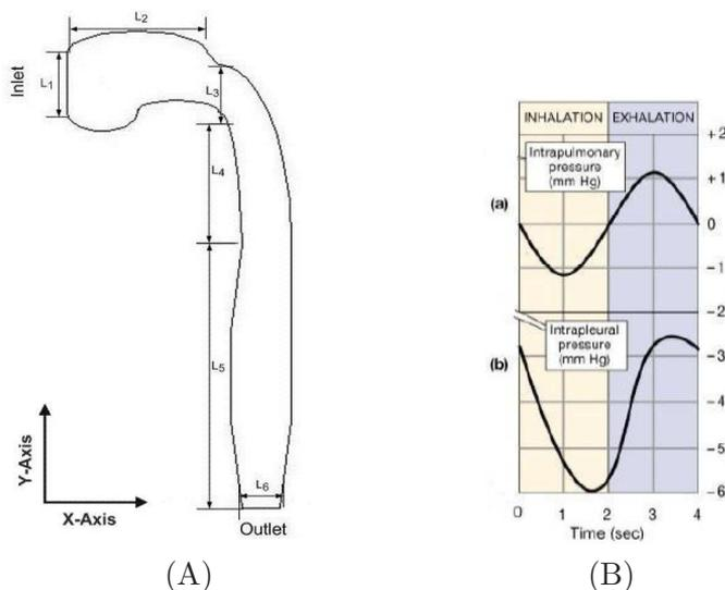
Figure 1: (A) 2-D respiratory tract model; (B) graphs of (a) intrapulmonary and (b) intrapleural pressure(modified from [17])
