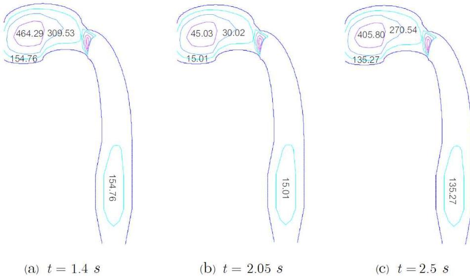
Figure 6: Contour plots of the airflow field( $cm/s$ ) in the respiratory tract model
