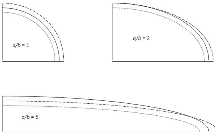
Figure 2: Schematic illustration of relation between initial ellipse (dotted line), free ellipse (broken line) and equilibrium ellipse (full line), at different aspect ratio
