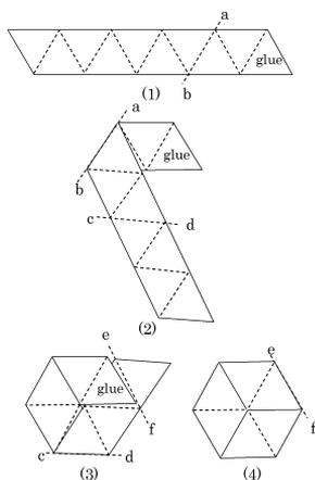
Figure 11: 3-face folding template and folding method
