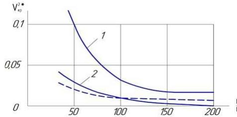
**Figure 2:** Dependence of the dimensionless critical velocity of the load on the relative thickness of the shell
