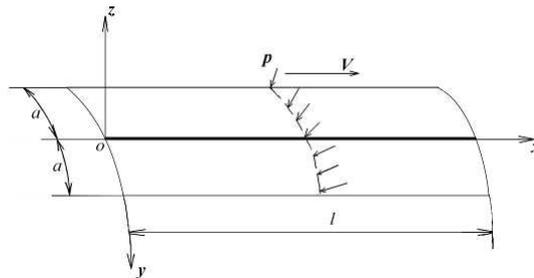
**Figure 1:** A sloping panel of a cylindrical shell
